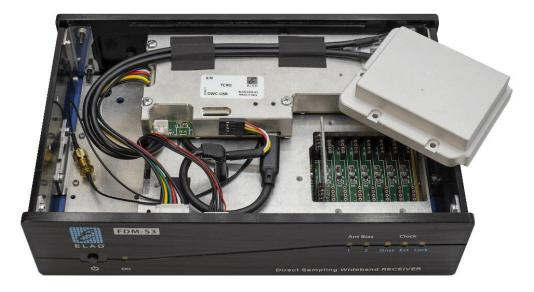
To change the preselector filters configuration remove the top cover of the FDM-S3 and the preselector filters shield as shown in the picture above. Insert the desired filters, take note of filters positions and then replace the shield and the cover.
